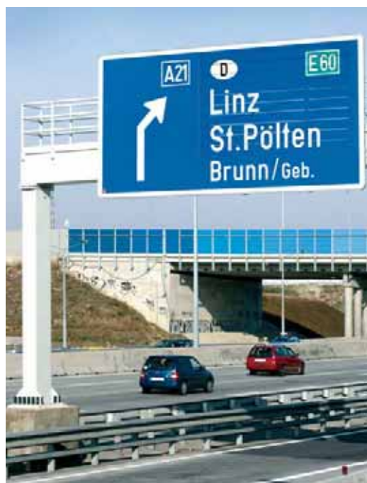
Some 1000 m 2 of type 3 DG sheeting and antidew overlay film were applied to the overhead signs.
